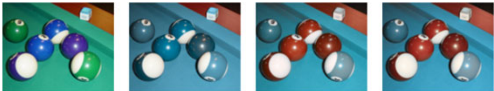
Figure 5. Rasche et al [12] proposed algorithm: From left to right: a natural image and the natural image as seen by a tritanope; a recolored image using the Rasche et al. algorithm and the recolored image as seen by a tritanope. Image taken from [12]
